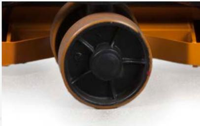
Polyurethane steer wheels and load rollers
