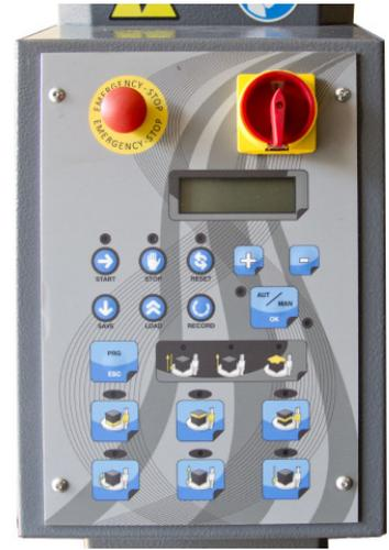
**Adjustable parameters by the control panel:** cycle selection, bottom turns, top turns, rotation speed, carriage speed going up, carriage speed going down, film tension.
